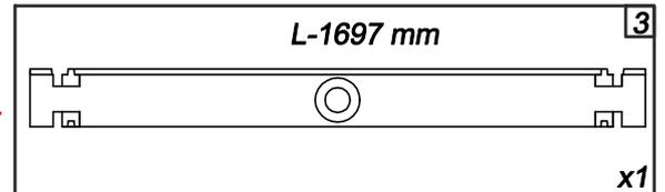
**(GB)** Install the beam no 3 on the 4th layer. If pool installed in area where temperatures fall below 0°C, install the beam no 3 on higher layer.
