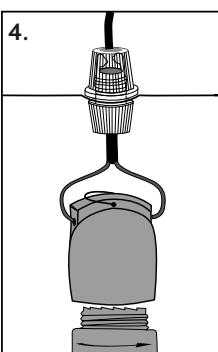
When installing the lamp with a clamp fixture, ensure that the lamp is fixed securely. The lamp must not be attached to pipes!
